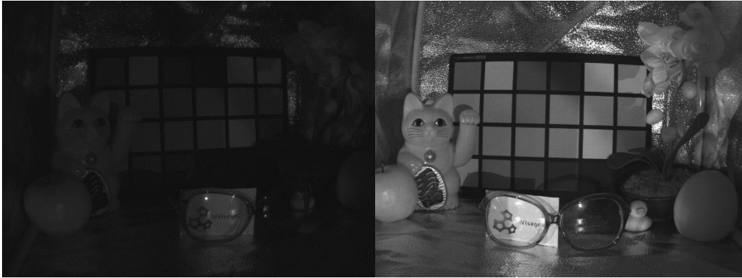
Figure 7. Comparison images taken with Spark4K with QuantumFilm and a silicon-based 13-megapixel (1.1 \mu\text{m} pixel size) image sensor. The 940 nm LED pulse durations were 10 ms in both cases.
