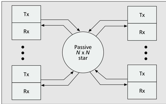
■ Figure 1. A fiber optic CDMA network using a passive  $N \times N$  star coupler.
