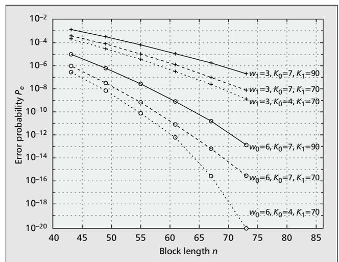
■ Figure 4. Error probability as a function of block length  $n$  for the multiple-weight MWOOC. The two code weights are  $w_0 = 6$  and  $w_1 = 3$  [8].
