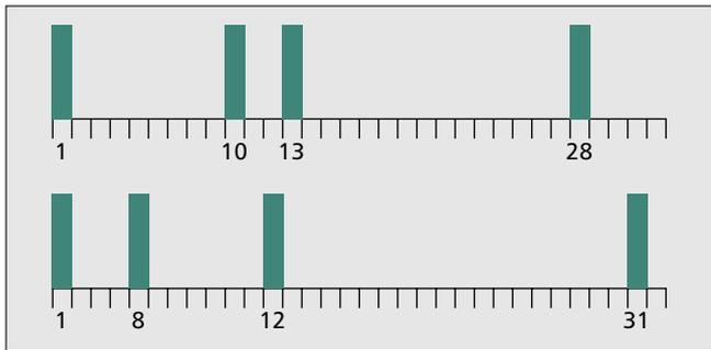
■ Figure 2. Two optical orthogonal codes with length  $n = 32$ , weight  $w = 4$ , and autocorrelation and cross-correlation constrained to one.
