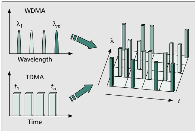
■ Figure 3. A graphical representation of WDMA, TDMA, and multiple-wavelength optical CDMA. TDMA and WDMA only take advantage of a single degree of freedom (time and wavelength, respectively). The multiple-wavelength optical CDMA scheme spreads data in both the time and wavelength domains to achieve greater flexibility and eliminate centralized network control.
