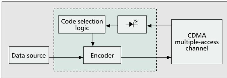
■ Figure 5. A dynamic encoder that adjusts the signature sequence based on the total network traffic.
